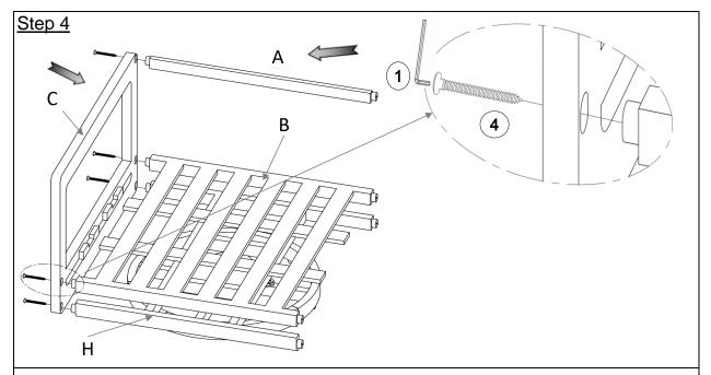
With assistance from you adult partner, attach Left Leg Panel (C) to Seat Panel (B), Plate (H) and Backrest (A) by using Screws (4) with Allen Wrench (1) as shown above.
