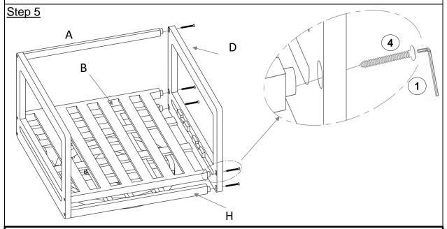
With assistance from you adult partner, attach Right Leg Panel (D) to Seat Panel (B), Plate (H) and Backrest (A) of the assenbled part in Step 3 by using Screws (4) with Allen Wrench (1) as shown above.
