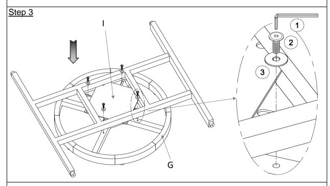
With assistance from you adult partner, attach the assembled part in Step 2 to Swivel Base (G) by using Screws ((2)) and Washers ((3)) with Allen Wrench ((1)) as shown above.
