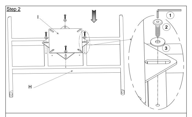
With assistance from you adult partner, attach Swivel Plate (I) to Plate (H) by using Screws (2) and Washers (3) with Allen Wrench (1) as shown above.
