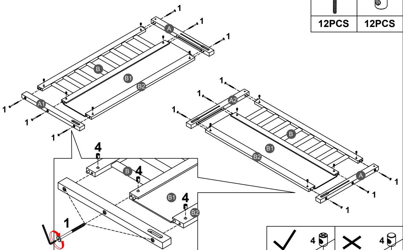
Note: Part 4 will face up with the "x" mark on it, otherwise it cannot be tightened
