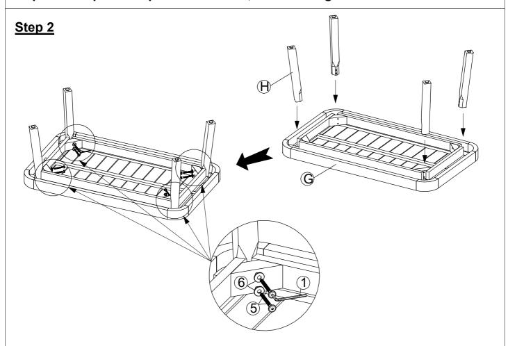
Attach Leg (H) to Top Table (G) by using 2 Bolts ( ) and 2 Washers ( ) with Allen Wrench ( ) as shown above picture.
