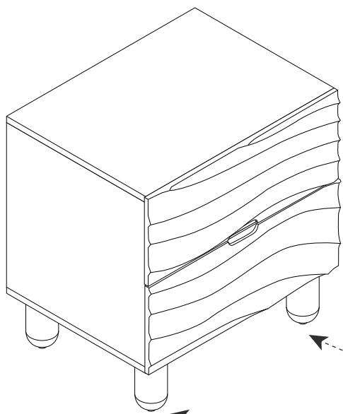
Note: Turn the feet adjusters to level up the unit.
