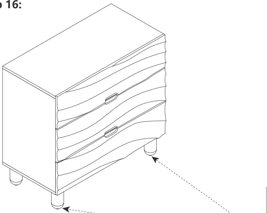
Note: Turn the feet adjusters to level up the unit.
