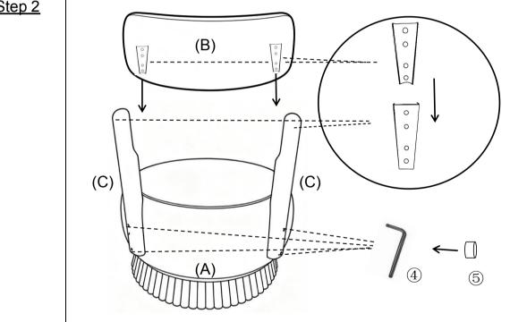
Please insert the sofa backrest (B) onto the already assembled support rod (C) and secure it firmly. Then use the allen key(4) to tighten the assembly from step 1.
