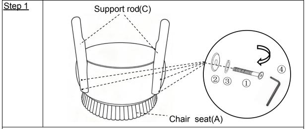
Place the chair seat(A) steadily on the soft carpet, position the support rod(C) against the chair seat(A) aligning the mounting holes, and connect them using the bolt (1), flat washer ring (2) and spring washer (3). tighten with the allen key (4).
