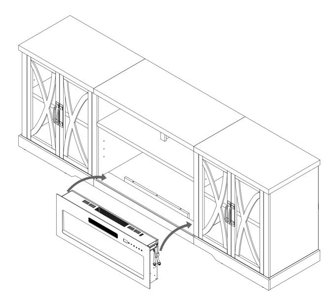
Place the electric fireplace into the wooden cabinet from the front. For instructions on using the electric fireplace, please refer to the electric fireplace manual.
