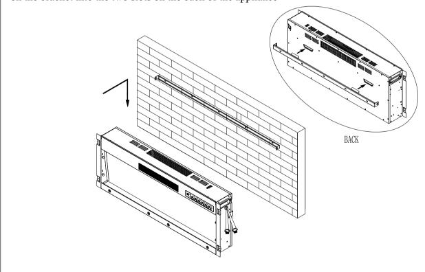
E.Use original screws to fasten wall bracket, Install the crystal.
