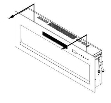
C.Place the electric fireplace in the wooden cabinet from front to back and fix the electric fireplace to the wooden cabinet with 4 screws.
