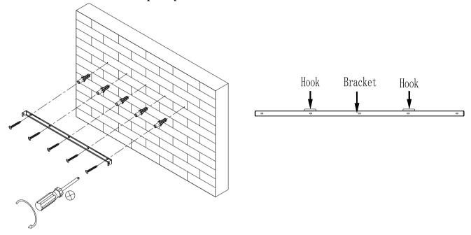
D. With the wall mounting bracket installed have two people lift the appliance up and insert the two hooks on the bracket into the two slots on the back of the appliance
