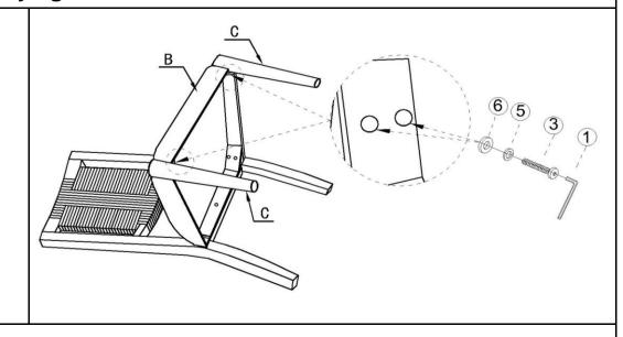
Install the Legs (C) using the Allen Wrench (①), Bolts (③), Spring washers (⑤) and Flat washers (⑥), as pictured above.
