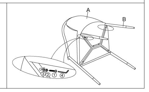
Using Bolt(①), Spring Washer(②), Washing Ring(③) With Allen Wrench(④) to fix Back Leg(B) to the Seat and Backrest(A) as shown above.
