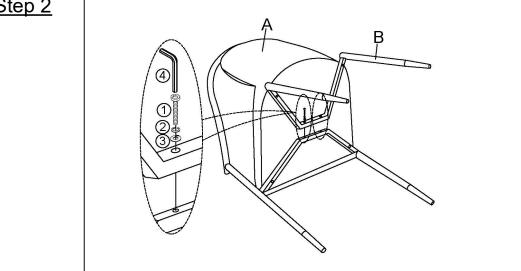
Attach Back Leg(B) to the Seat and Backrest(A) using Bolt(1), Spring Washer(②), Washing Ring(③) With Allen Wrench(④) as shown above. After all Bolts are in place, use Allen Wrench(4) to tighten Bolts on Back Leg(B) fully.
