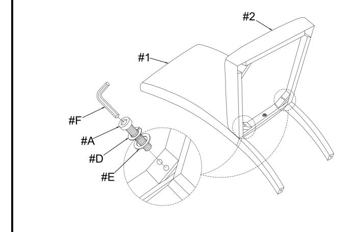
Do not tighten screws until completely asembled.
