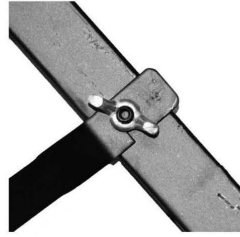
**Step 3.** Tighten the wing nut until secure. Repeat the same process for all four end legs, making sure all wing nuts are tightly secured.
