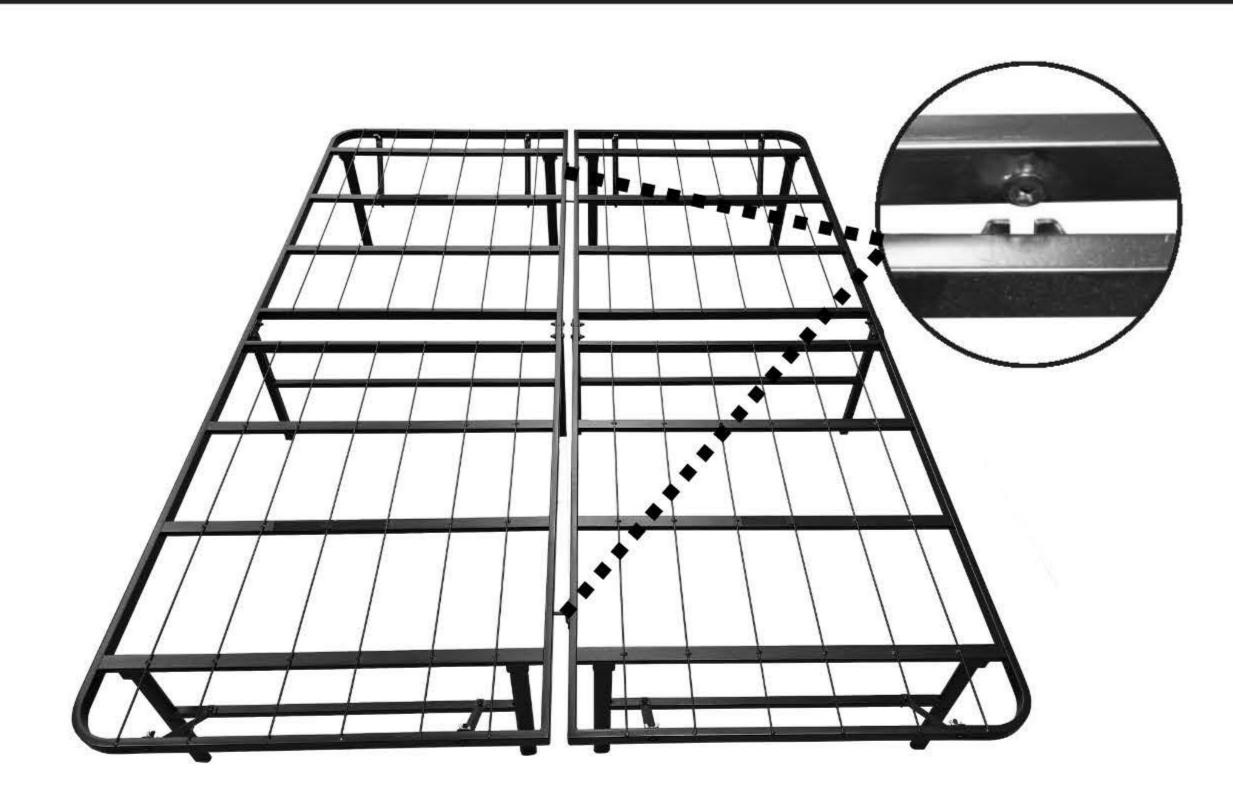
**Step 5.** Insert two halves together with keyhole locked in place.
