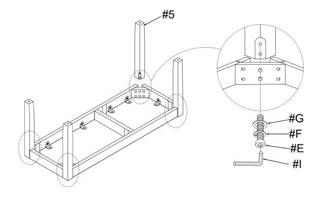
Do not tighten screws until completely asembled.
