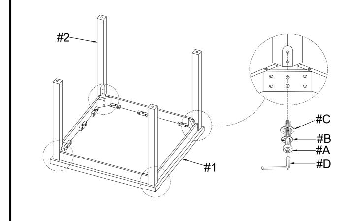
Do not tighten screws until completely asembled.
