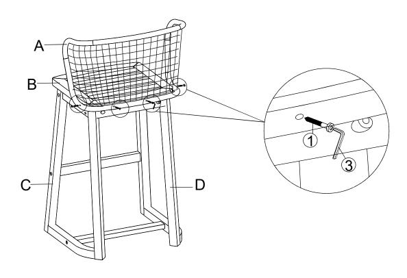
Attach Backrest Frame (A) into the Seat Panel (B) by using Screws (1) and Allen Wrench 3.
