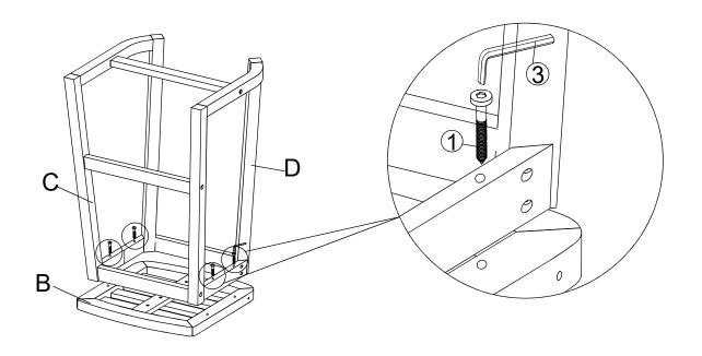
Place the Seat Panel (B) on the clean , non-marring surface. Secure the assembled frame in step 3 to the Seat Panel (B) by using Screws (1) and Allen Wrench (3).
