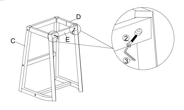
Attach Back Support Bar (E) into the Right Leg Panel (C) and Left Leg Panel (D) by using Screws (2) and Allen Wrench 3.
