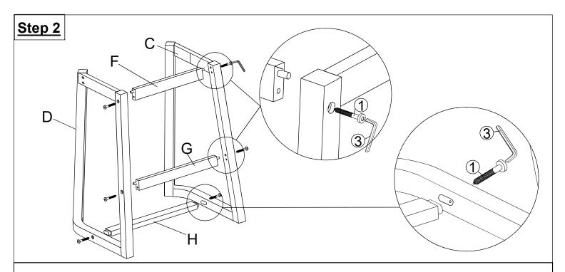
Attach Front Support Bar(F) ,Upper Support Bar (G), Lower Support (H) into the Right Leg Panel (C) by using Screws ( $\widehat{1}$ ) and Allen Wrench  $\widehat{3}$ . Repeat the same process for the Left Leg Panel (D).
