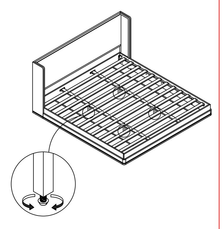
Rotate counterclockwise to increase the length of Floor Leveler, and raise that corner. Rotate clockwise to lower that corner.
