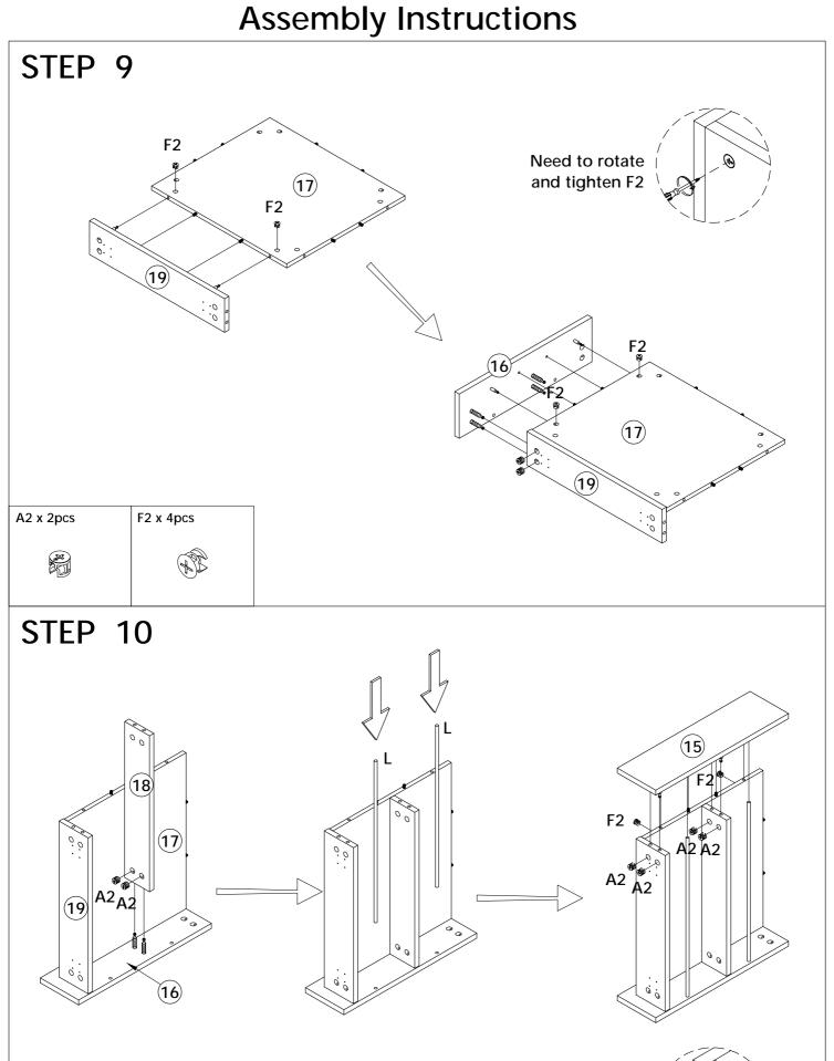
Need to rotate and tighten F2
