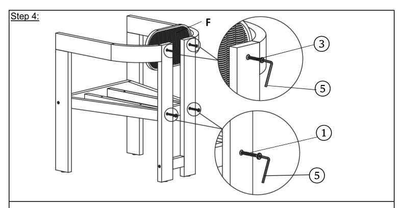
With the help of your adult partner, secure Seat Frame (E) to Leg Panels (A, B) by using Screws (1) with Allen Wrench (5).
