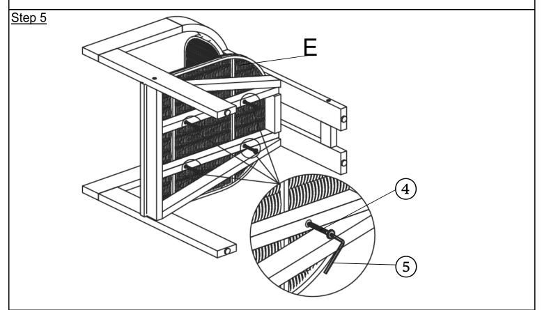
With the help of your adult partner, turn the assembled part in Step 4 left side down as shown above then secure Seat Panel (E) to Seat Frame (C) by using Bolts (4) with Allen Wrench (5).
