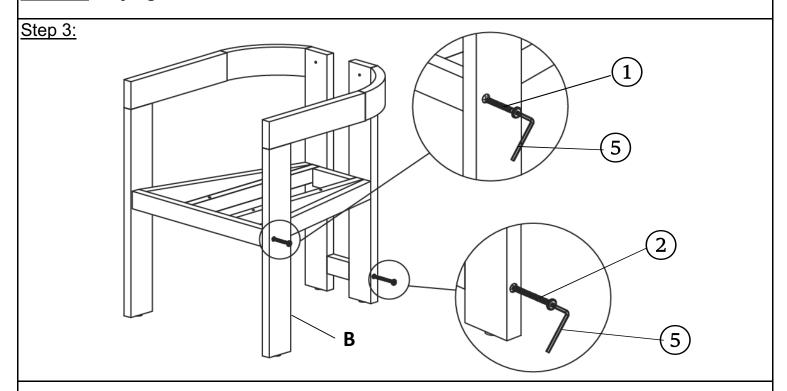
With the help of your adult partner, insert the tenons of Seat Frame (C), Leg Support Bar (D) of the assembled part in Step 2 into the mortises of Right Leg Panel (B) as shown above. Secure Right Leg Panel (B) to Seat Frame (C) by using Screws (1) with Allen Wrench (5). Secure Right Leg Panel (B) to Leg Support Bar (D) by using Screw (2) with Allen Wrench (5). **DO NOT** fully tighten the Screws.
