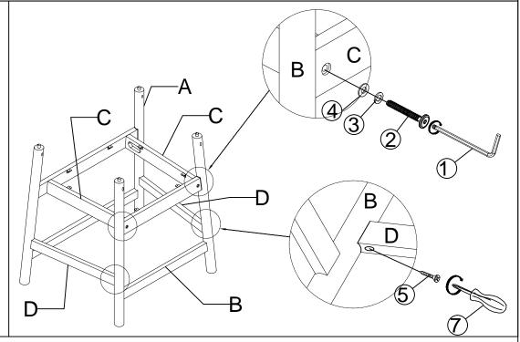
Connect the Rear Leg Frame (B) into the Front Leg Frame (A) using the Allen Wrench (1), Bolts (2), spring washer (3),
