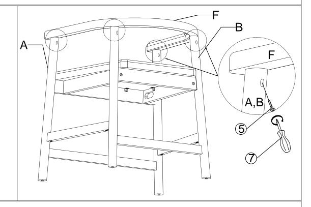
After connecting the backrest (F) to the frame is completely installed with Screw (5) and Screwdriver (7) Tighten the Screw.
