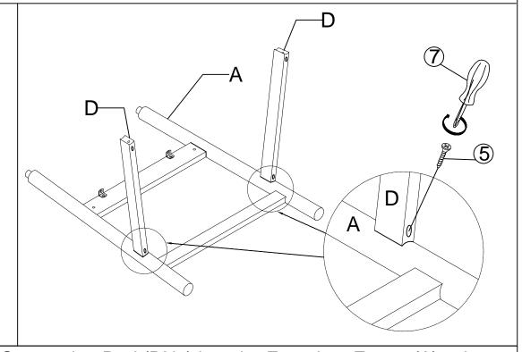
Install the Connecting Rod (DX2) into the Front Leg Frame (A) using Screwdriver (7) and Screws(5). Tighten the Screws.
