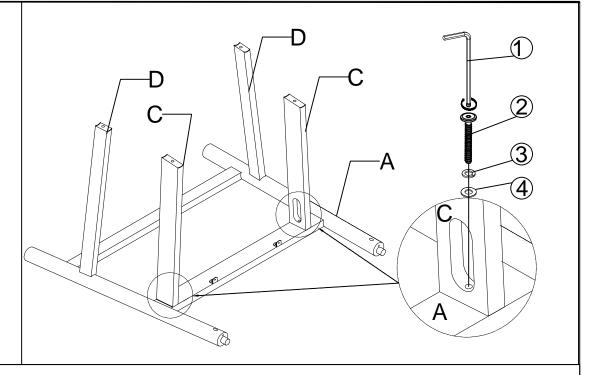
Install the Support Frame (Cx2) into the Front Leg Frame using the Allen Wrench (1), Bolts (2), spring washer (3), flat washer (4). Tighten the Bolts.
