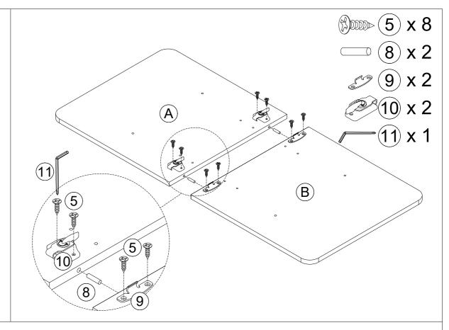
Attach metal latch( ) to top board(A) with screw( ),attach metal latch( ) to top board(B) with screw( ). Insert metal bar( ) to connect with top board(A) and top board(B) using allen  $key(\widehat{\mathbb{1}})$ .
