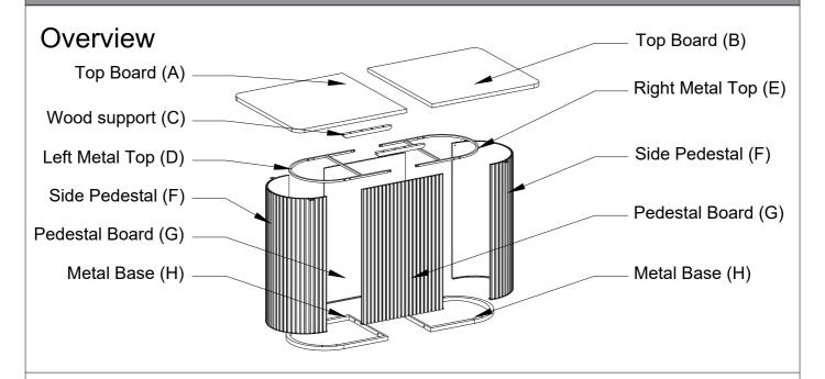
This counter table has multiple parts and may require up to some 30 minutes to assemble. To give you an overview of the counter table parts, the above picture is to help you put the various parts into perspective. Please read through the instructions below to familiarise yourself with the parts and steps before assembly.
