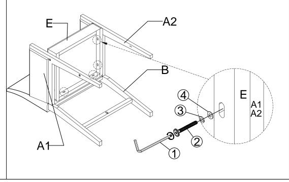
Install the Seat cushion (E) into the Left, Right Side Leg Frame(A1, A2) and Rear Leg Frame(B) using the Allen Wrench (1), Bolts (2), spring washer (3), flat washer (4). Tighten the Bolts.
