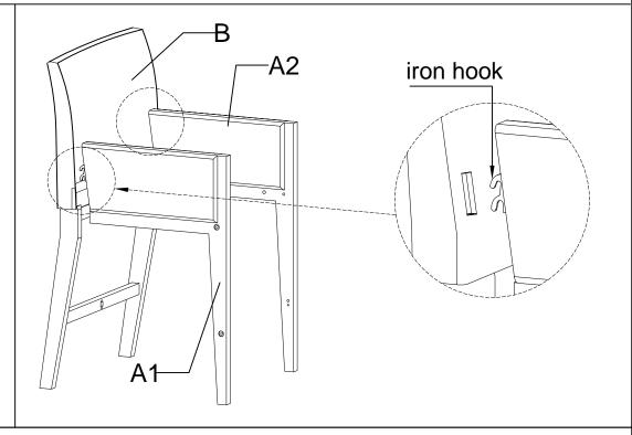
Install the Left, Right Side Leg Frame (A1,A2) into the Rear Leg Frame (B) by iron hook
