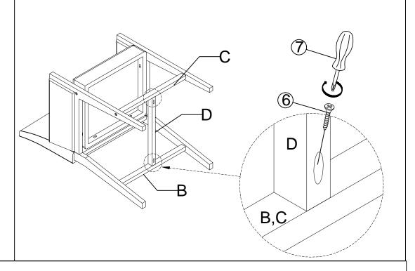
Use the Screwdriver (7) and Screws (6) to connect the Vertical connecting Rod (D) with Horizontal connecting Rod (C) and Rear Leg Frame(B). Tighten the Screw.
