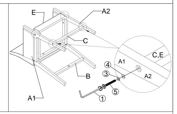
Connect the Left, Right Side Leg Frame(A1, A2) with the Horizontal connecting Rod (C) and Seat cushion (E) using the Allen Wrench (1), Bolts (5), spring washer (3), flat washer (4). Tighten the Bolts.
