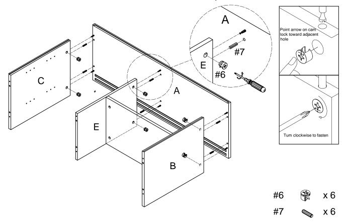
Step 6. Attach bottom panel (part D) to assembled unit (parts B, C & E) using tapping bolts (part #4), wood dowels (part #7) and allen wrench (part #14).
