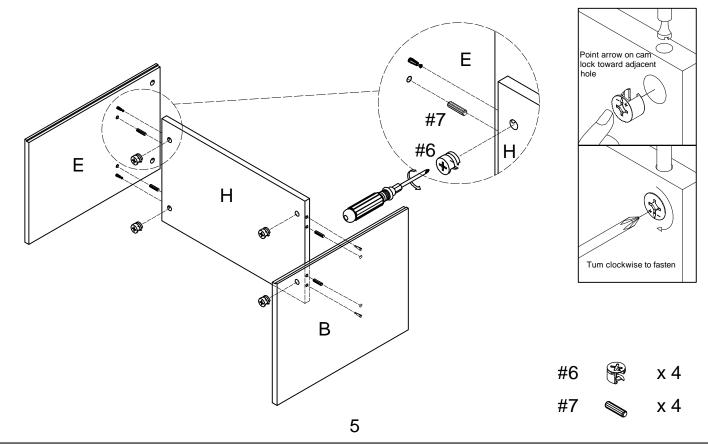
Step 5. Attach panels (parts B, C & E) to top panel (part A) using cam locks (part #6), wood dowels (part #7) and phillips head screwdriver.
