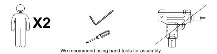
If an electric screwdriver is used, reduce power and torque to avoid damage to the product.
