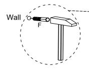
If it is a solid wall, please use expansion and self-tapping screws, if it is a wooden wall, only use self-tapping screws, please do not overtighten the screws
