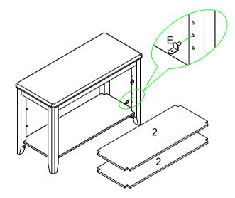
Note: Attach hardware E to the foot columns as illustrated, and then place the No. 2 movable laminate in the position indicated.
