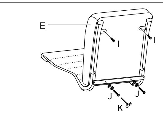
**Step 4**: Attach Seat **E** with Assembled Seat Back via Screws **Ix2** and Screws **Jx2** as shown in the picture and finish with Allen Wrench **K**.
