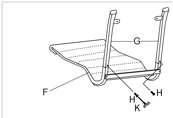
**Step 3**: Fix Brackets **Gx2** with the Chair Back **F** with Screws **Hx2** and finish with Allen Wrench **K**.
