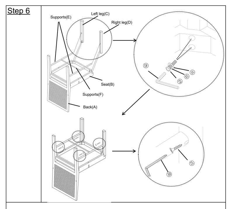
6.1)Attach the Legs(C+D) into the Seat(B)using bolts(②),Spring washer(⑥) and Washer(⑧) with Allen wrench(⑨).
