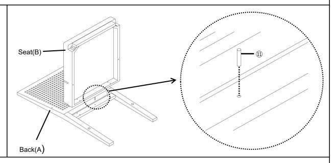
Slot the wood plug(1) into the position hole on the Back(A) and slot another end of wood plug into the position hole of Seat(B),as shown bove.
