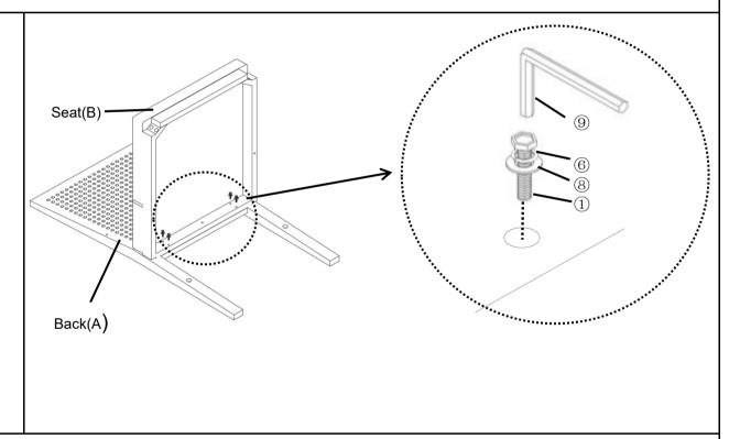
Attach the Seat(B) into the Back(A)using bolts(①),Spring washer(⑥) and Washer(⑧) with Allen wrench(⑨).
