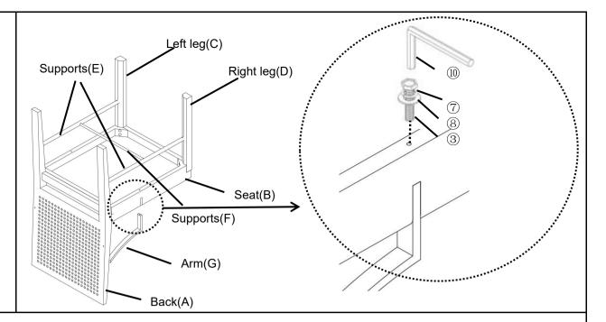
Attach the Arms(G) into the Seat(B)using bolts(3),Spring washer(7) and Washer(8) with Allen wrench(10).
