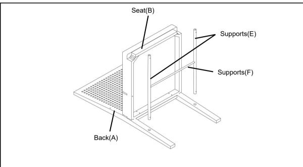
Insert the Support(E) into the mounting positions of the Back(A).
