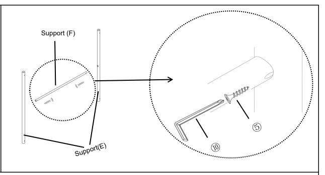
Insert the Support(F) into the mounting positions of the Supports(E) using Screws(5), with the Allen wrench(10).
