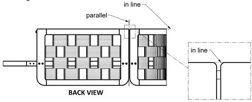
Use the Allen Key (HW2) to screw in 2 of the bolts (HW1) on the side of the seat panel (C) as shown. Do not fully tighten.
