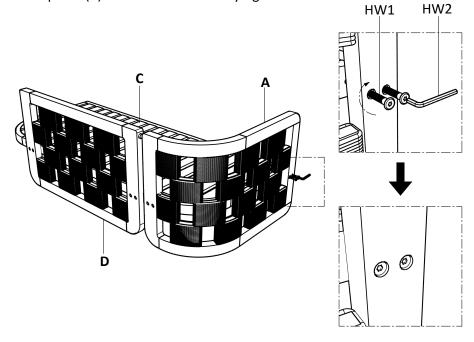
Align the screw holes on the right side panel (B) to the screw holes on the seat panel (C) and insert the dowel guide on the back panel (B) into the dowel hole on the right side panel (A). Use the Allen Key (HW2) to screw in 2 of the bolts (HW1) on the back of the seat panel (C) as shown. Do not fully tighten.
