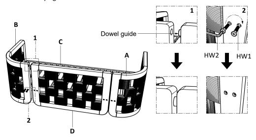
Before tightening the bolts, the 2 side panels must be in line with each other. Once they are in line, then tighten the bolts
