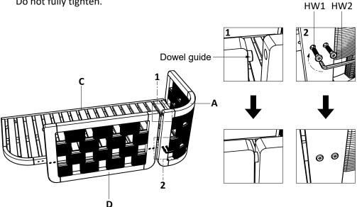
Before tightening the bolts, the 2 side panels must be in line with each other. Once they are in line, then tighten the bolts.
