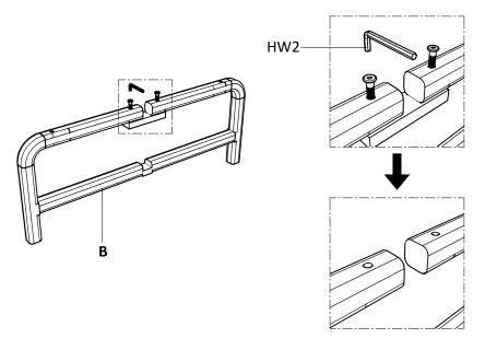
Insert Leg 1 (B) into Leg 2 (C) as shown below.
