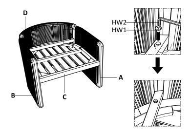
Turn the chair upright. Open the webbing near the posts of the back panel (D). Use the Allen Key (HW2) to screw in 4 of the bolts (HW1) into the 2 posts as shown below. Fully Tighten all the bolts.
