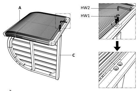
Align the screw holes on the right side panel (B) to the screw holes on the seat panel (C). Use the Allen Key (HW2) to screw in 2 of the bolts (HW1) near the front of the seat panel (C). Do not fully tighten.
