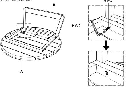
Align the screw holes in the second leg (B) to the screw holes underneath the top table (A). Use the Allen Key (HW2) to screw in 4 of the bolts (HW1). Fully tighten all the bolts.
