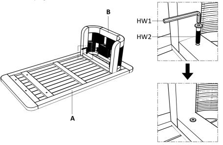
Align the screw holes in the second leg (B) to the screw holes underneath the top table (A). Use the Allen Key (HW2) to screw in 4 of the bolts (HW1). Fully tighten all the bolts.
