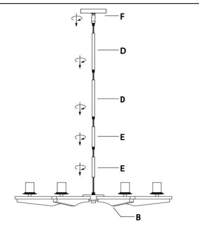
Step 2: Screw the Long Stem (D) and Short Stem (E) to the Lamp Body (B). Make sure to feed the branch wires of the fixture through the stems during assembly. Remove or add stems to adjust the height. Then screw the canopy (F) to the stem.
