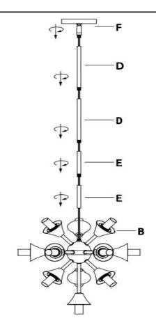
**Step 2**: Screw the Long Stem (D) and Short Stem (E) to the Lamp Body (B). Make sure to feed the branch wires of the fixture through the stems during assembly. Remove or add stems to adjust the height. Then screw the canopy (F) to the stem.
