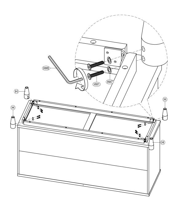
Turn the unit upright and adjust the levelers on the bottom of the legs as needed.
