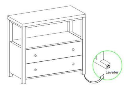
Leveller are provided at the bottom to the balance on uneven suface
