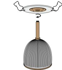
**Step5**: Align and rotate clockwise the Marble top (E) on Pipe (B).
