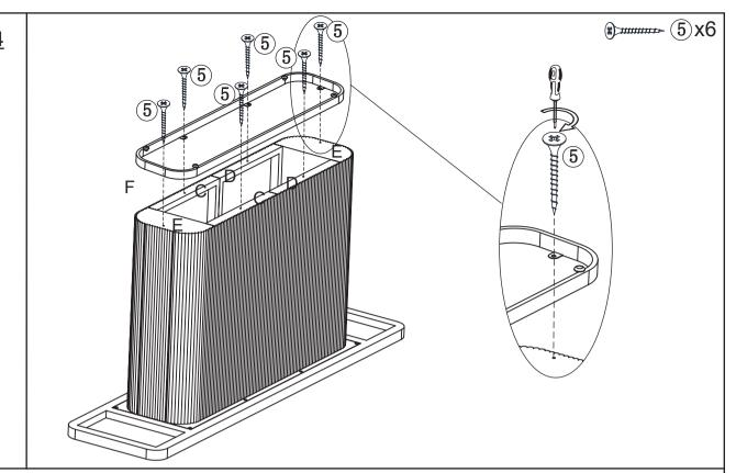
Attach the leg (E) and the panel 2&3(C,D) to the metal base ring (F) with screw(\$).
