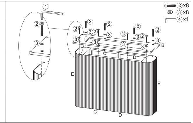
Attach the leg (E) and the panel 2&3(C,D) to the panel 1(B) with bolt(2) and flat washer(3) using allen wrench(4).
