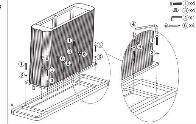
Attach the top panel (A) to the panel 1(B) with bolt(1) and flat washer(3) using allen wrench(4). Attach the top panel (A) to the panel 1(B) with screw(6).
