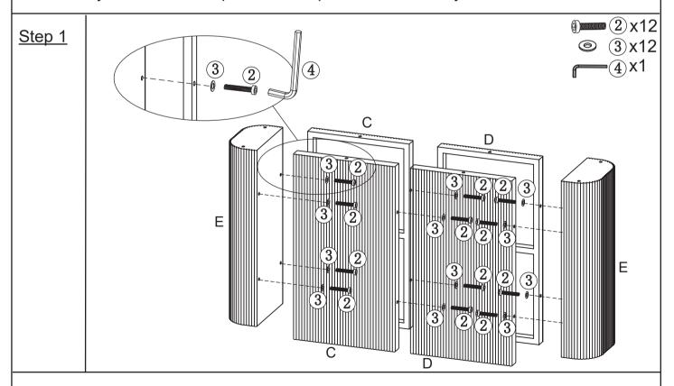
Attach the panel 2&3(C,D) to the leg (E) with bolt(②) and flat washer(③) using allen wrench(④).
