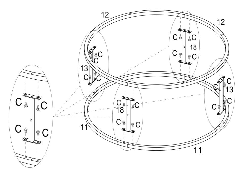
As shown in the figure, assemble the curved steel pipes 11 and 12 into a circle, then use steel pipes 13 and 18 to connect the two circles vertically.
