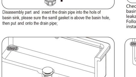
Tighten the fasten nut by hand;
