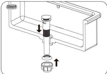
At this step, small gasket is not needed, please follow the step 2 and step 3 to complete installation.
