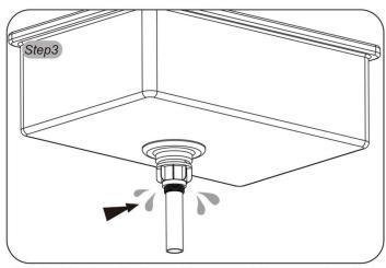
Check whether leakage happened here under the basin sink; You need apply some silicone to prevent leakage issue if there is leaksge under the basin sink, Follow steps 4 to apply the silicone and complete installation;
