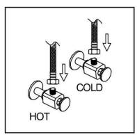
5. Attach flexible hose to water supply.
