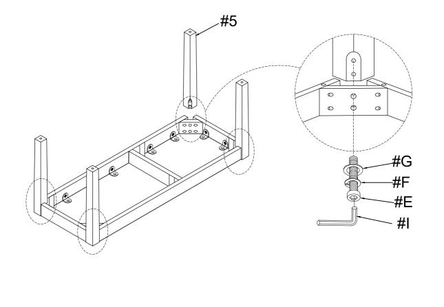
Do not tighten screws until completely asembled.
