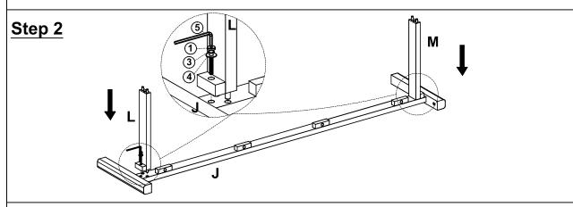
Place the Front Leg Frame (J) and the Left Support Rail (L) and the Right Support Rail (M) on a carpeted surface. Attach the Support Rail (L),(M) to the Front Leg Frame (J) using Botl ( 1) and Lock Washer ( 3) and Flat Washer ( 4) with Allen Wrench ( 5) as shown in the picture.
