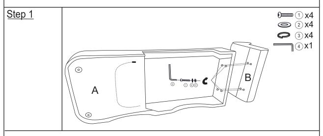
Place the seat base(A) upright on the floor. Align the four inner holes of the backrest(B) with the four holes on the lower part of the backrest.Install and tighten the screws.
