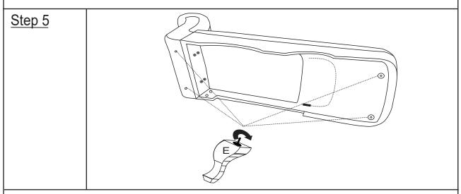
Place the ottoman on its side and attach the ottoman legs(E) to the bottom.
