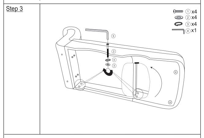
Unzip the bottom of seat base (A) to locate the two inner holes. Align the four circled holes in the diagram with the four holes on the lower part of left back (C). Insert and tighten the screws from the inside.
