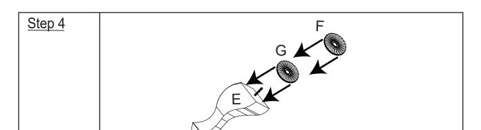
Place the rubber flat gasket(G) onto the screw of the ottoman leg(E) then place the plastic flat gasket(F) onto the rubber flat gaskert(G).
