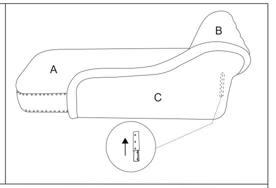
Insert the tab from the left back (C) into the backrest (B)'s tab from bottom to top.
