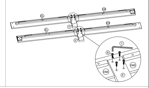
Attach the Side Rail-Left (DL&EL) and Side Rail-Right (DR&ER) to Side Rail Leg (F) by using Bolts (⑥) with M4 Allen Wrench (①).
