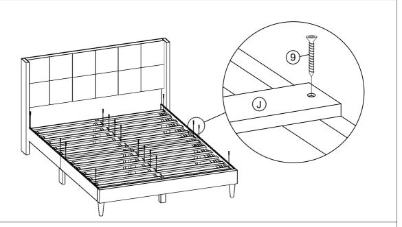
Attach all Slats (J) to the rail on Side Rail (D&E) by using Screws (9) and Screwdriver (Not Provided).
