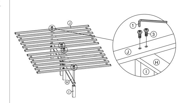
Attach the Center Leg (I) and Bed Slats (J) to the Center Rail (H) by using Bolts(③) with M4 Allen Wrench (①).
