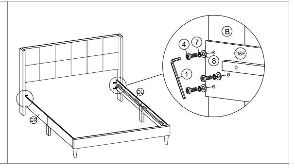
Attach the Assembled Side Rail (D&E) to Headboard Side (B) by using Bolts (4), Spring Washer (7), Flat Washers (8) with M4 Allen Wrench (1).
