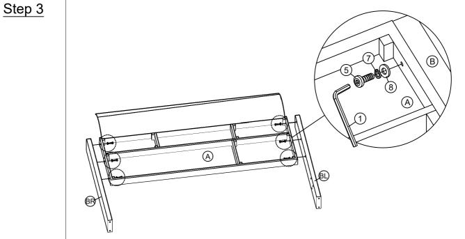
Attach the Headboard Side (BL&BR) to Headboard (A) by using Bolts (⑤), Spring Washer (⑦), Flat Washers (⑧) with M4 Allen Wrench (①).
