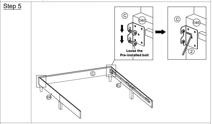
Loosen the bolts slightly on the Footboard (C), then attach the assembled Side Rail (D&E) to the assembled Footboard (C), tighten the bolts using with M5 Allen Wrench(2).
