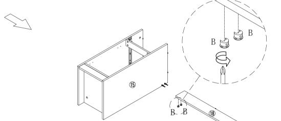
Make sure the arrow on the screw align to the hole on the side. put B on board 18 B\*2
