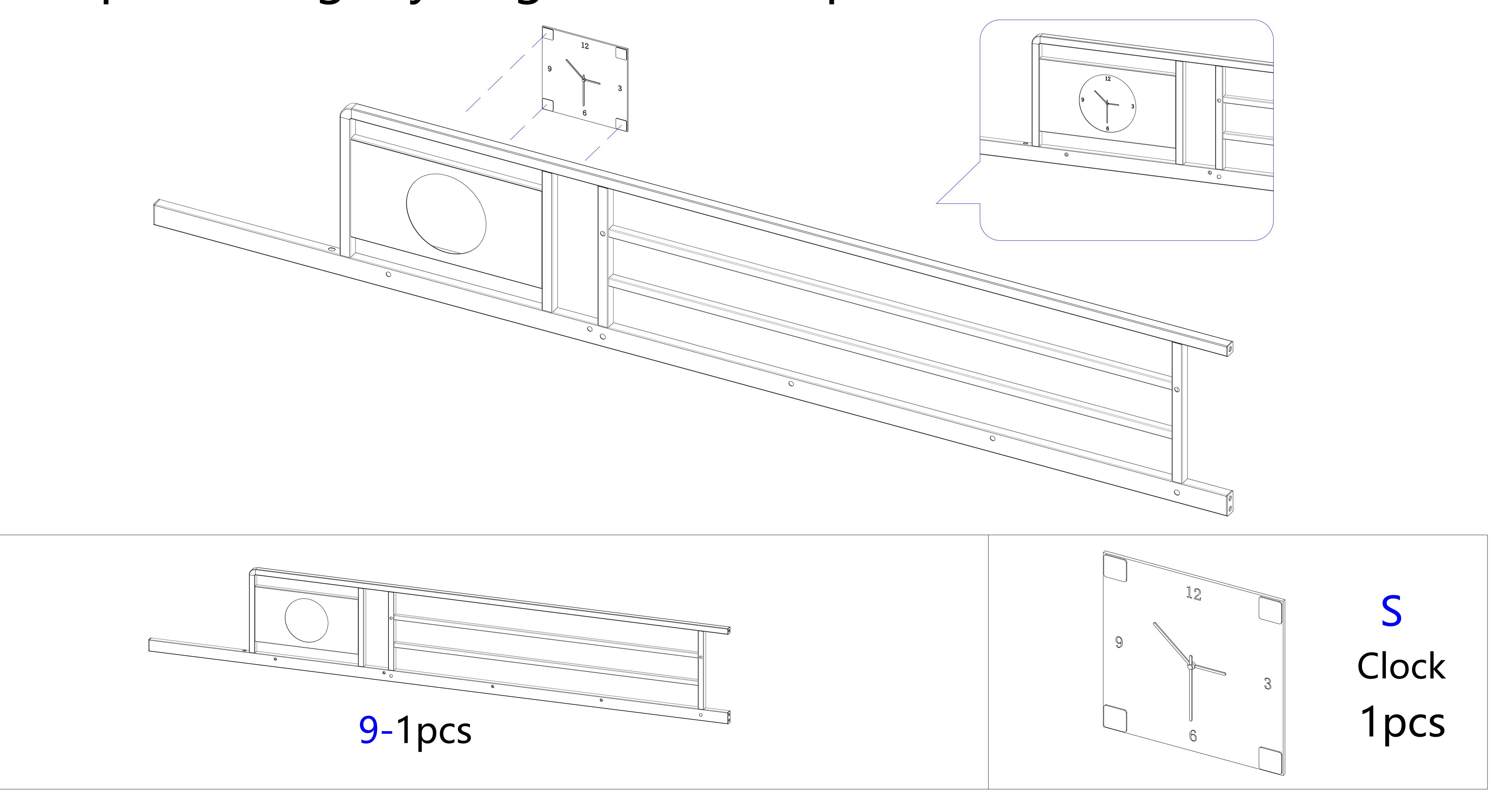
Step 3: Use hardware L,Q,A,B,T,Y,C to connect #1 #4 #15 #16 #14 and #9 component together.
