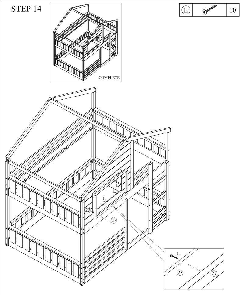
Attach the door frame (27) to the panel (23) using the pre-drilled holes as shown.
