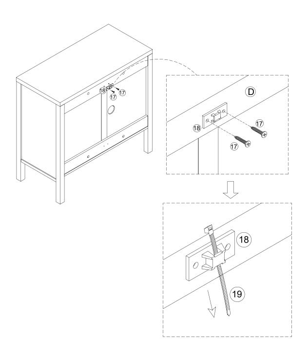
Find where you want your storage unit to live and then mount the Plastic Bracket (18) to the wall using the provided Wall Anchors (20) and M4\*35mm Screws (21). We recommend using a 1/4" drill bit.
