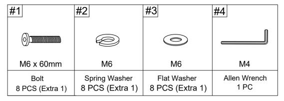
Step 1. Lay table top (part A) upside down on a soft surface, such as carpet. Attach legs (part B) to table top (part A) using bolts (part #1), spring washers (part #2), flat washers (part #3) and allen wrench (part #4).
