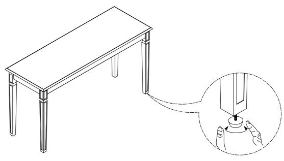
Note: It is important to adjust levelers once fully assembled and upright.
