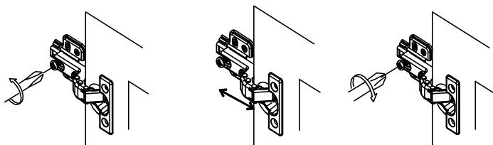
This is used to adjust the door panel in the front and back direction: Loosen the screw first, and then tighten screw after adjusting the door panel to the proper position.
