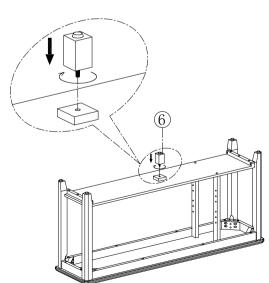
► As shown in the figure, align Component No. 6 with the reserved hole at the bottom of step 2 and tighten it with the nails in a timely manner
