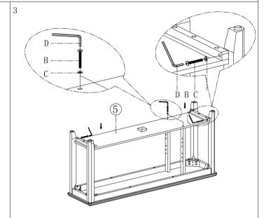
► As shown in the figure, assemble Component No. 5 with Step 1 using part B/C/D
