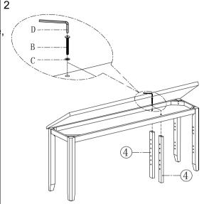
► As shown in the figure, assemble components 4 using parts B/C/D. 。
