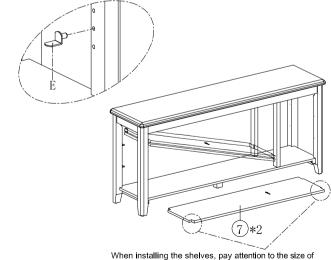
When installing the shelves, pay attention to the size of the notches on both sides. The larger side is on the left side of the schematic diagram
